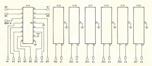
Fig. 7. Memory address select M0–M9 are tied to all seven memory chips as is the memory Read/Write command (MEM W). All chip enable ( $\overline{CE}$ ) pins must be tied to ground.
